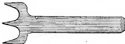
Gauge for Marking Positions of Studs in Upholstery.
